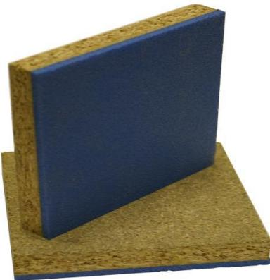
**Karma Overlay 23** is a high performance acoustic floor panel with an exceptional performance to height ratio. Comprising an 18mm tongued and grooved 18mm P5 chipboard to a 5mm cross linked polyolefin foam resilient layer. Karma Overlay 23 provides excellent impact and airborne sound insulation in a single product. It is used on an existing floor, new ply or chipboard floor or directly to concrete/screed floors making it an ideal product for refurbishments and new build projects.
